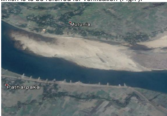
Fig.No.8. The spur locations and probable effect of currents at right embankment (source: google earth)
